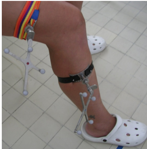
Fig. 1: The position of the passive markers fixed to the patient's tibia and femur.
