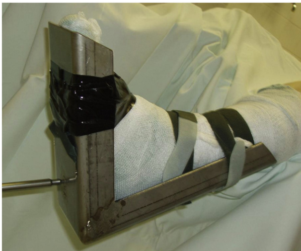
Fig. 1. “Iron shoe” mounted to the cadaver foot providing 100°dorsal flexion in the tibio-talar joint.
