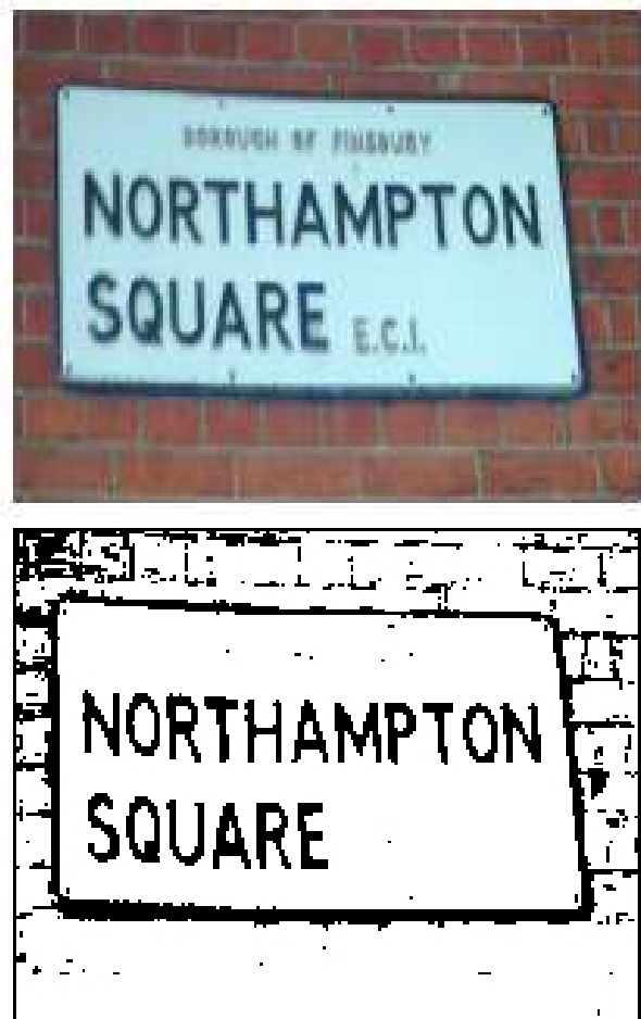
Figure 5: Pattern recognition of road signs: (a) original image; (b) detected image
