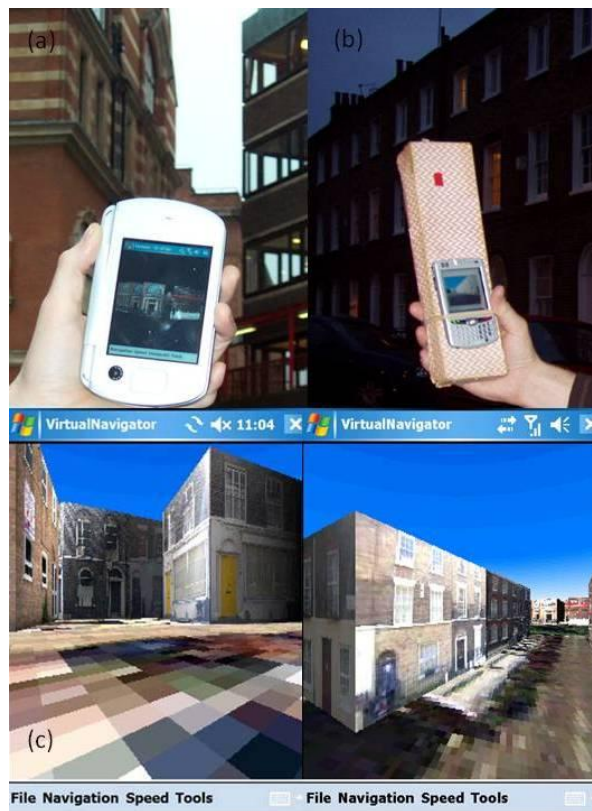
Figure 3-2 Mobile VR Interfaces (a) Manual mode (b) GPS mode (c) VR view
