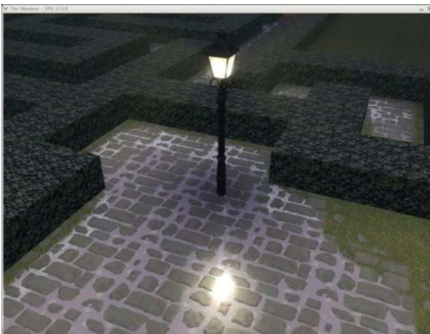
Fig. 8 Achieving a mirror effect by rendering the geometry twice (Anderson and McLoughlin 2007)
