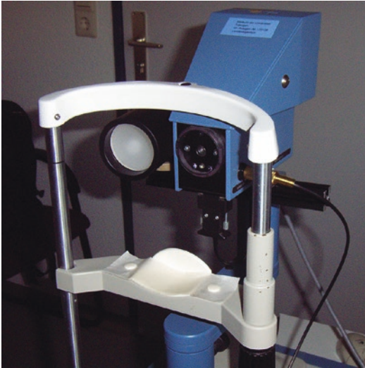
Fig. 7.6 Chromatic pupilligraphy equipment in our laboratory. The stimulus is provided by a mini-Ganzfeld color LED stimulator to one eye and the consensual pupil light reflex of the nonstimulated fellow eye is measured by the compact integrated pupillograph (AMTech GmbH, Dossenheim, Germany)
