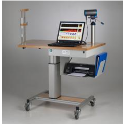
Fig. 6 PSTxsIII Pupillographic Sleepiness Test (AMTech, Germany). Recording the spontaneous and involuntary pupil movement in darkness is the simplest method to measure and evaluate sleepiness objectively. The sleepiness waves are monitored by means of a IR-videocamera with built-in IR-illumination. The subject is bespectacled with a pair of goggles which are opaque for visible light and transparent for infrared light. Thereby the measurement is performed in darkness and only a crimson and dim fixation target is seen. The Pupillographic Sleepiness Test is an easy to operate, non-invasive and fast tool to obtain an objective assessment of the central nervous activation and drug related vigilance. Areas of application are sleep medicine, occupational medicine and pharmacology ( www.amtech.de ).
