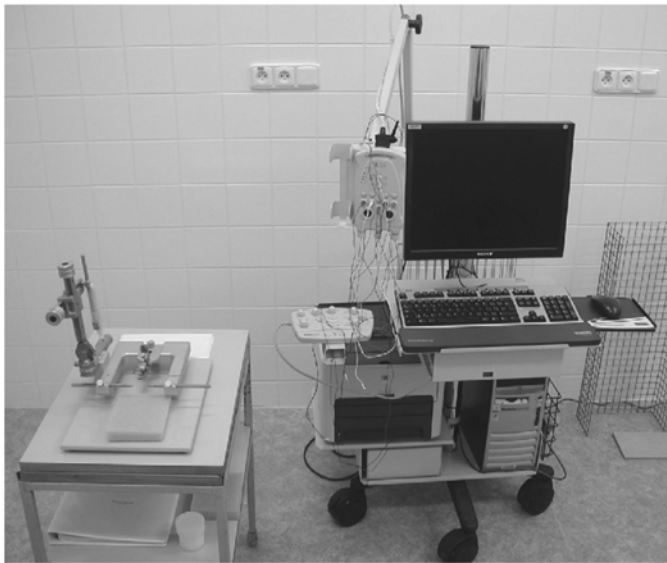
Fig. 6. Electrophysiological device connected to a computer (right) with a stereotaxic holder (left).
