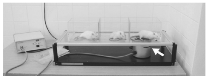
Fig. 1. A plantar apparatus (Ugo Basile, Comerio, Italy) which measures the hind paw withdrawal latency from a radiant heat source (arrow). Note that three rats can be tested in one session.
